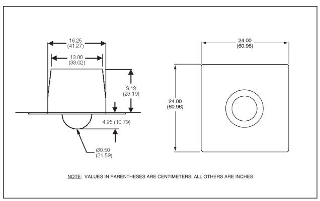
Figure 7. BB08A120 Dimension Drawings
